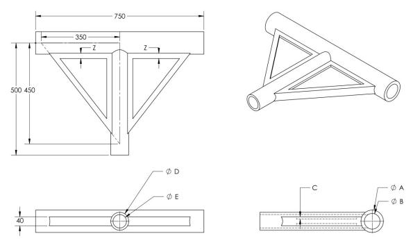
Create the part in Solidworks, using the following values for the given variables. Use the unit system MMGS, and Alloy Steel (density = 7700 kg/m^3). The cutouts on the webs are on both sides (there should be 4 total).
